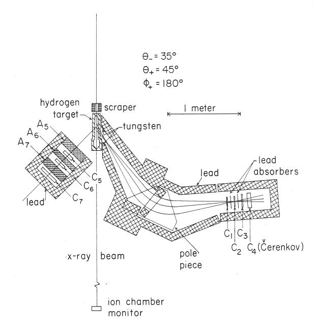
Using the magnetic spectrometer alone, data was also taken of the  $\pi^-$  production at 35° for several pion energies and several bremsstrahlung cut-off energies. The cross-section for  $\pi^-$  production was deduced from the measured rates by the method described in the work of Bloch and Sands (20, 21).
