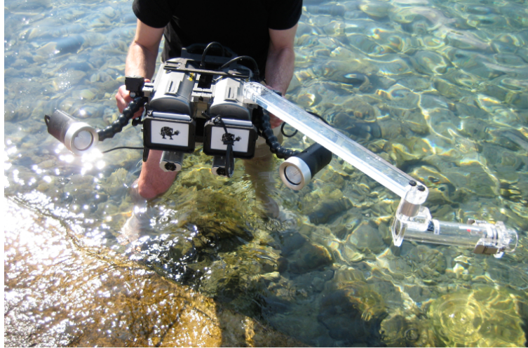
Figure 6.1. The most recent design iteration of SCUVA incorporates two video camera housings separated by a fixed distance with multiple-level HID lights, which allows for the capture of three-dimensional particle trajectories.
