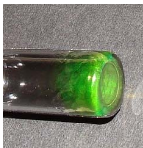
Figure 13. Photograph of slowly dried g\text{-}[\text{PLA}_{200}\text{-}b\text{-}Pn\text{BA}_{200}] (Table 2, entry 10) showing green color due to reflectance from the large self-assembled domains.
