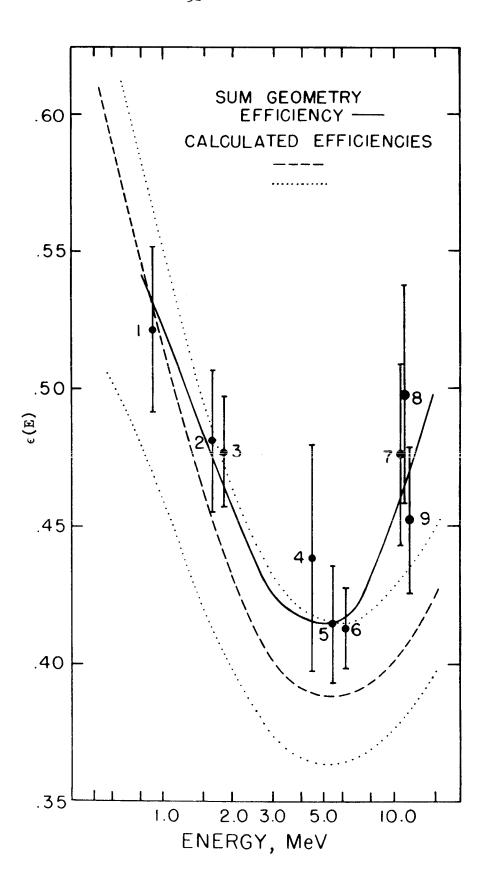
Also appearing in Figure 5 are the experimental data, and the solid curve through the data points represents the efficiencies adopted for the unmodified spectrometer. In view of the errors just discussed, the deviation of the solid curve from the envelope defined by the two dotted curves (which represent limiting cases) is not considered to be serious. The experimental points were determined in the following several ways.
