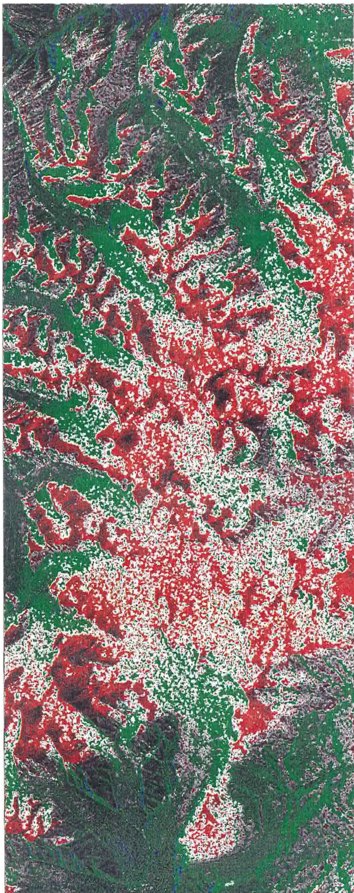
Figure 4.13 Regional C-band circular polarization ratio behavior in DT 1/58.10 Kumlun Mtn. scene. Color assignments are: red for \mu_c > 1.0 , green for 0.25 < \mu_c < 0.7 , and blue for \mu_c < 0.25 .
