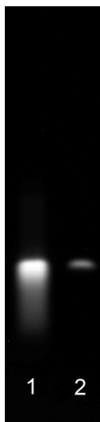
Figure 3-5: Lane 1 is our synthesized unlabeled DNA 20-mer without purification. Lane 2 is the HPLC purified unlabeled DNA 20-mer ordered from IDT
