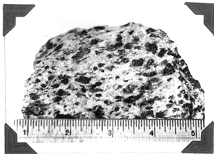
Hand specimen, S_{10R} , of the Parker quartz diorite showing gneissoid character of the rock. The black crystals are hornblende.
