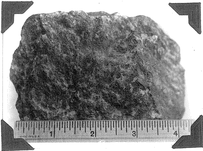
Hand specimen of quartz syenite. Dark material is largely biotite, white material is orthoclase perthite.
