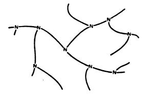
The PEI worked with had average molecular weights of 600 and 40,000. PEI (600) is an anhydrous liquid which is soluble in water (in all proportions) and other solvents such as DMF and methanol. The microanalysis is given below:
