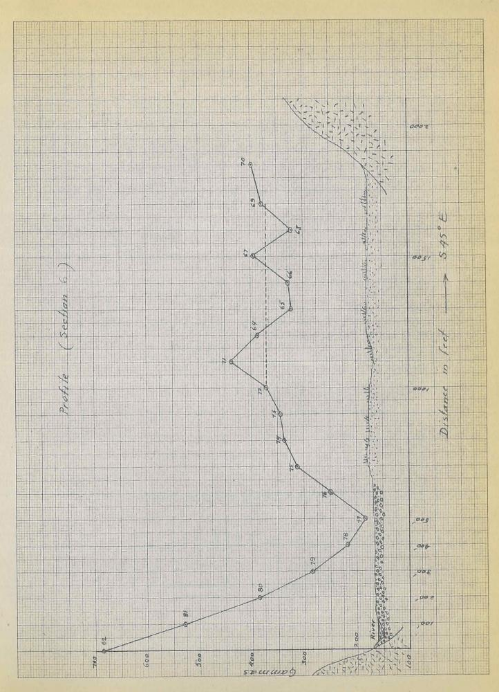
the soil-covered part, that is between 76 and 70, is about 370 gammas, whereas over the gravel wash it is 184 gammas. The sudden increase, starting over the gravel wash at Station 77, is due to the adjacent granite hill; otherwise it would be low over the channel (see Section 6).
