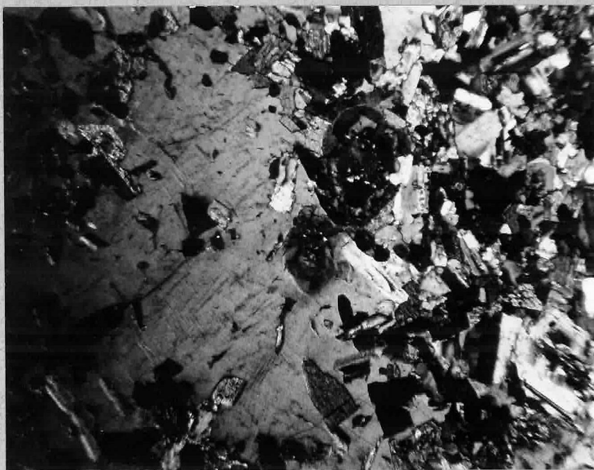
Figure 28B -- An enlargement of a part of fig. 28A showing residuals of hornblende, biotite and magnetite in the orthoclase of the granodiorite. Residual plagioclase also occurs but not within the field. (X40: crossed nicols)
