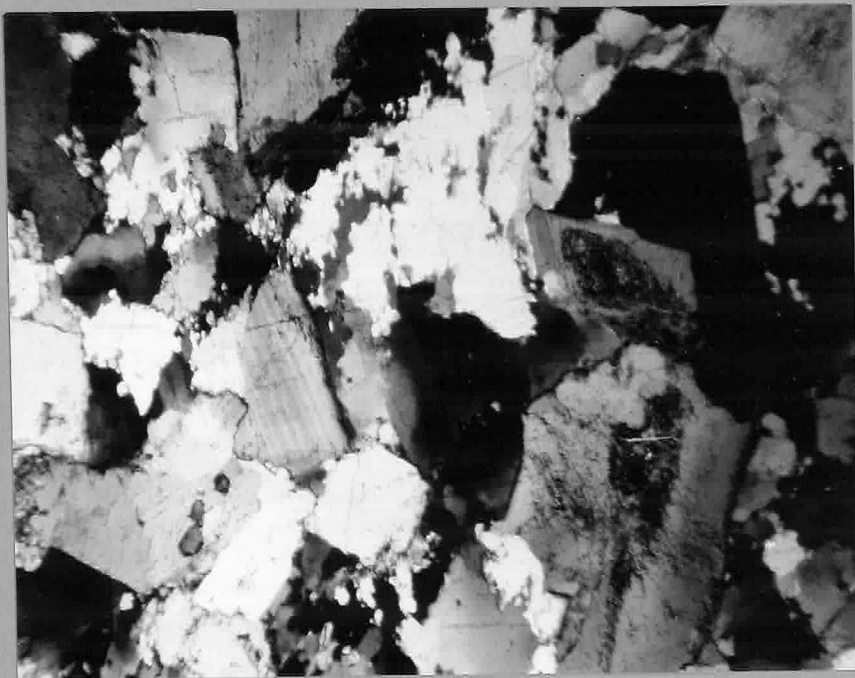
Figure 34 -- Sutured boundaries of quartz crystals in a specimen of Capilano quartz-diorite from the west base of Crown Mtn. It is, perhaps, suggestive of post-batholithic recrystallization. (X40: crossed nicols).
