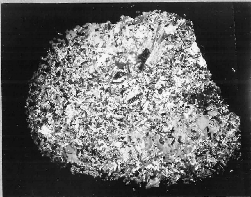
Figure 28A -- This depicts the random pervasion of calcic diorite inclusion by Hollyburn granodiorite. The granodiorite metacrysts contain inclusions of all the minerals comprising the diorite. Hornblende, however, is the most abundant residual (most of the diorite feldspar having been absorbed in the formation of the granitic metacrysts). (X5: crossed nicols)
