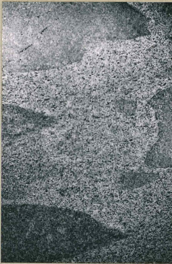
Figure 19 -- An illustration of "ghost" inclusions (especially right central portion of the photograph) in the Capilano quartz-diorite.
