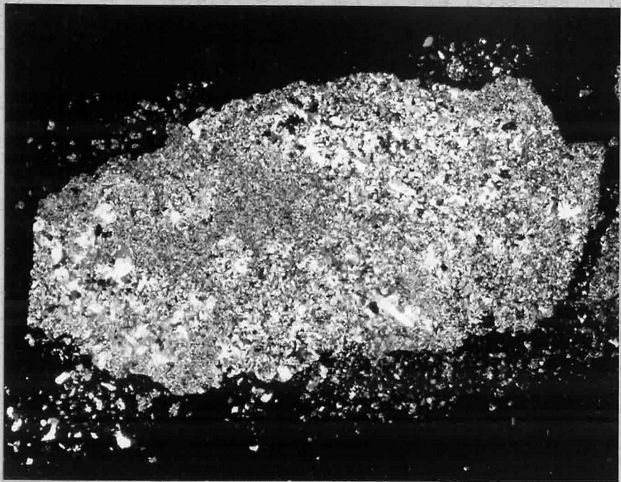
Figure 25A -- An irregular growth of granitic elements within a partly orthophyric (not well developed) fine-grained andesite. (X5: crossed nicols)
