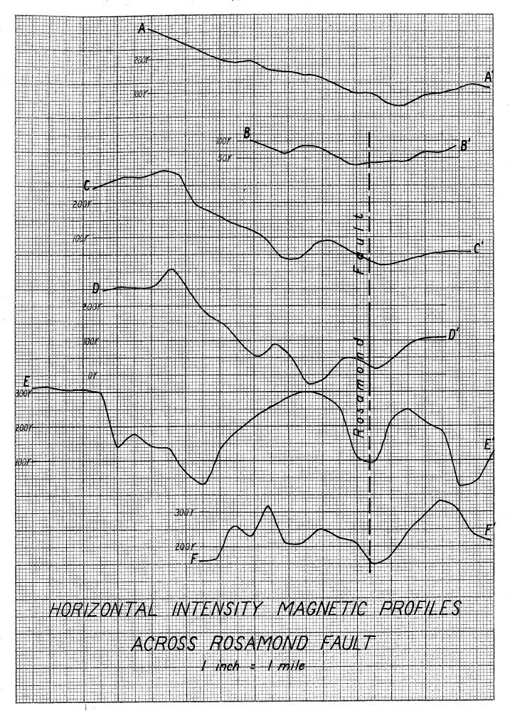
profile A-A' was run about a mile off the end of the fault as indicated on the map. It shows a general minimum at the line of the fault and might be interpreted to mean that the fault continues for a distance with decreased displacement. Profiles C-C' and D-D' show another minimum south of the fault. The significance of this anomaly is not known. Anomalies of large magnitude are present in the two eastern profiles, but their cause can only be a subject of speculation here.
