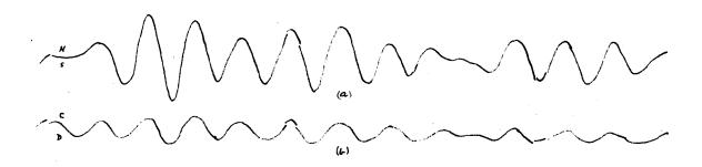
Part of seismogram of Panama earthquake of July 17, 1934 ( $a=42^{\circ}$ ), recorded by long period N - S Benioff seismograph ( $T_{0}=0.5$  sec.,  $T_{g}=13$  sec.) and b recorded by short period strain seismograph ( $T_{0}=0.014$  sec.,  $T_{g}=1.5$  sec.). These are surface waves arriving from the SE and are in phase. The record for the long period strain ( $T_{g}=28$  sec.) is identical with that for the short period strain for these waves.
