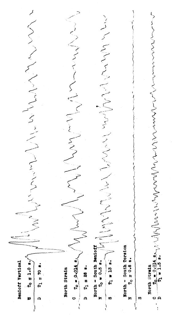
Tracing starts at 17h 44m 00s with a timing correction of #24 seconds. Part of seismogram of Panama earthquake of July 17, 1934 ( = 420), comparing the recordings on warious instruments.
