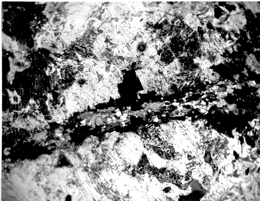
Fig. 40 Photomicrograph of vein in spotted diorite containing biotite (black), calcite (gray), and quartz (white), which is probably related to the alteration of the feldspars around the reaction rims.
