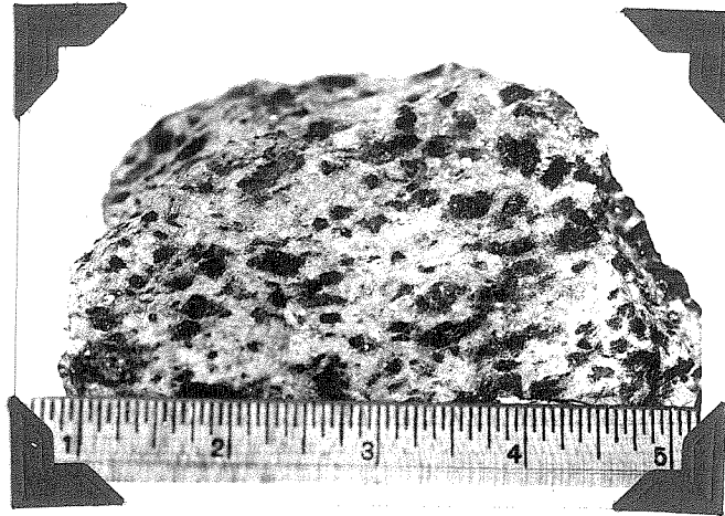
Fig. 27 --- Hand specimen of Parker Quartz Diorite. The dark masses are hornblende crystals, while the light-colored material is mostly albite and quartz. The albite is usually un-twinned.
