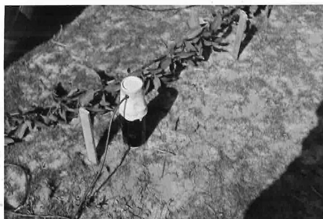
Figure 12. Potential electrode: asphalt coated porous clay pot with paper cap to keep the cable from twisting and to keep dust from the copper electrode and sulphate solution.
