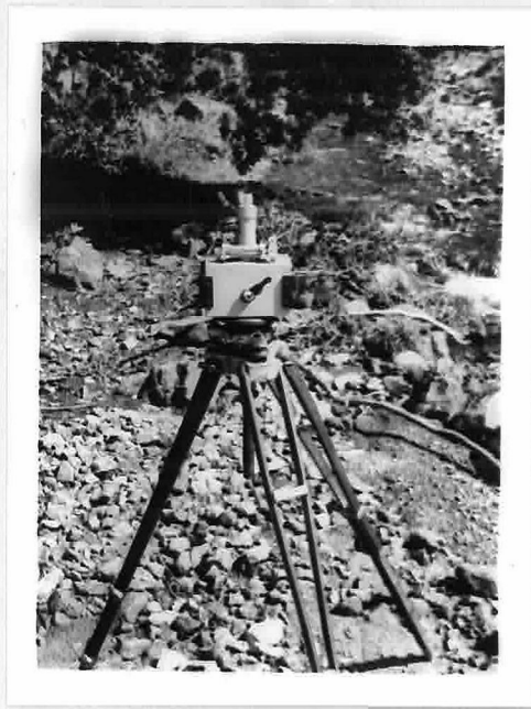
Fig. 2. The magnetometer as used in the survey.
