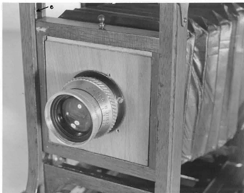
Figure 7 - Elgeet lens, 105 mm focal length, f 4.5, a series V adapter ring is attached to the rim of the lens. The f stop figures can be seen in the picture. Note the threads of the rise and fall screw (e).
