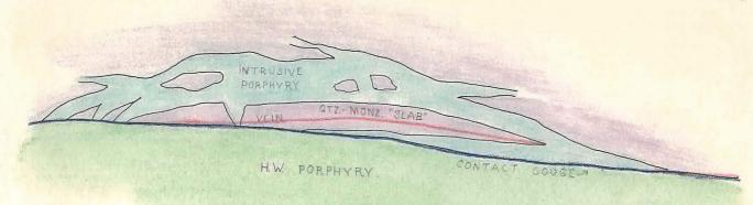
Generalized plan of the Cactus vein showing the porphyry intrusive and the isolated segment of quartz-monzonite. Scale: 1 = ±200 •
