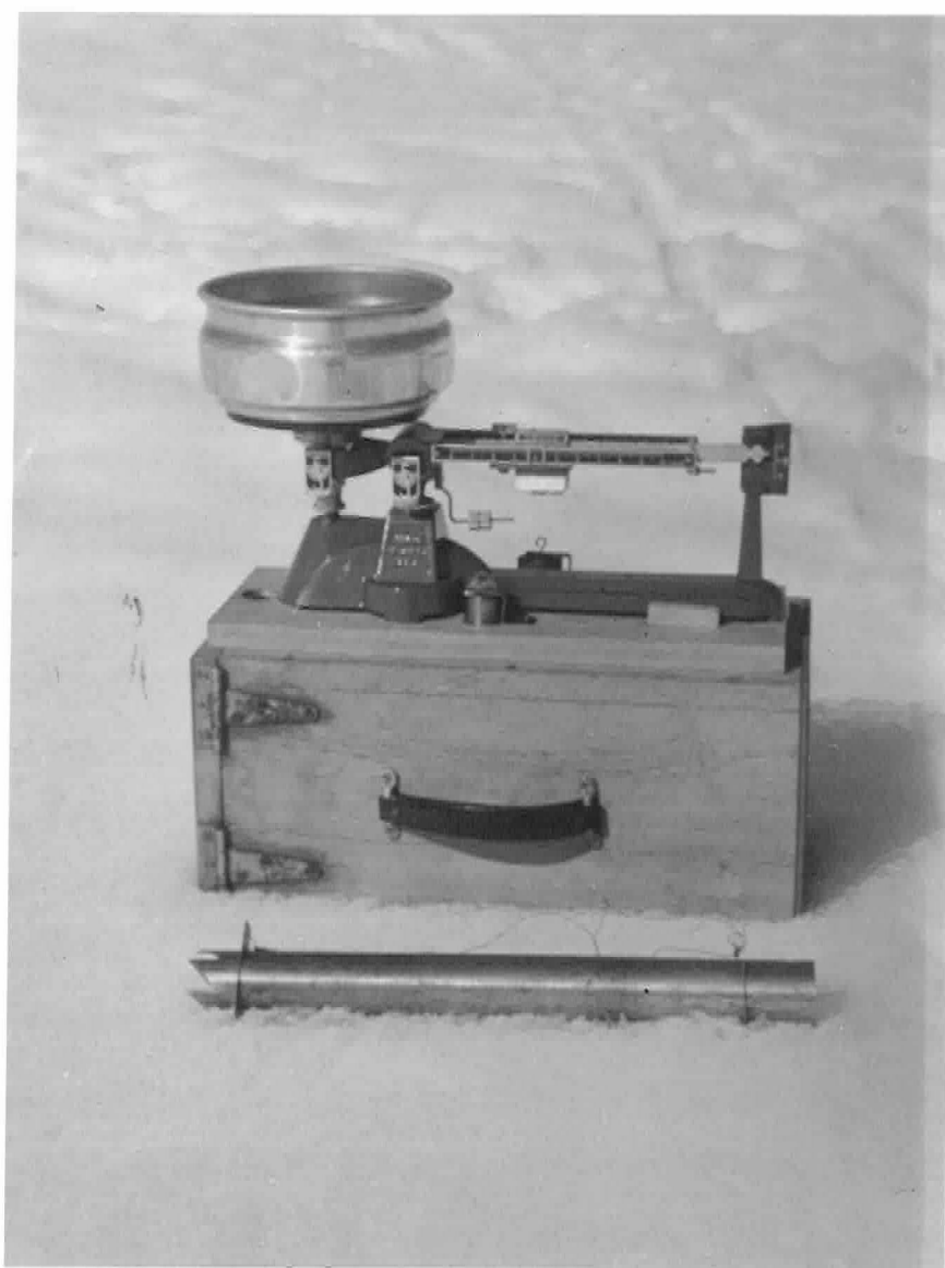
Fig. 7. Apparatus for measuring firn densities.
