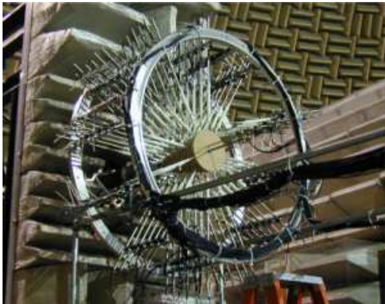
Figure 2.6: The Small Hot Jet Acoustic Rig (SHJAR) and Hydrodynamic Array at the NASA Glenn Research Center.
