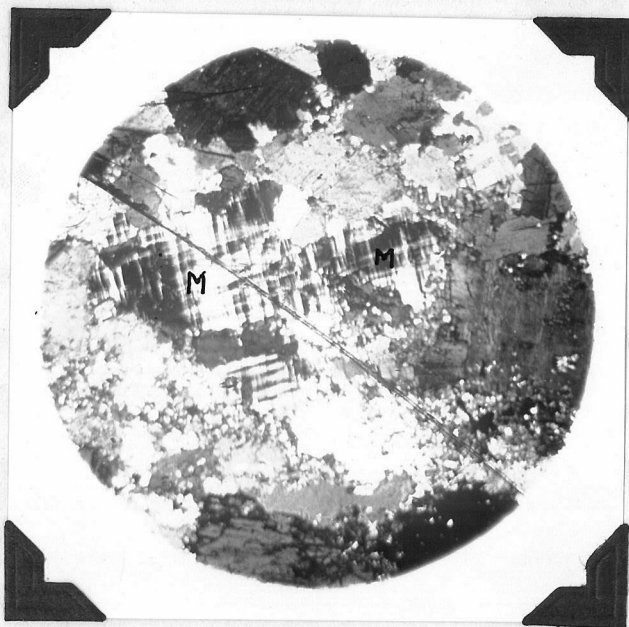
Figure 14 - Photomicrograph of Granite. X27. Crossed Nicols. (M) Microcline
