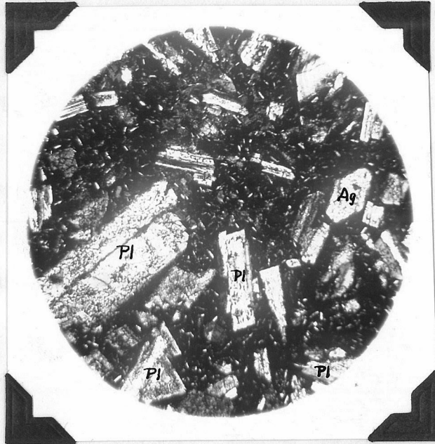
Figure 18 - Photomicrograph of Basalt. X27. Crossed Nicols (Pl) Plagioclase, (Ag) Augite.
