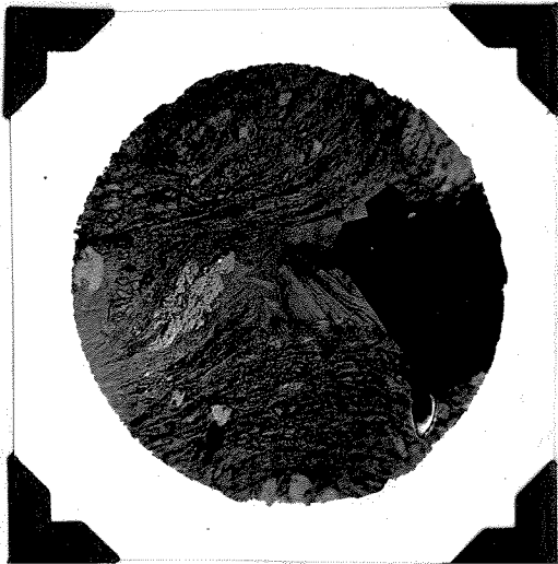
Figure 14. Chlorite orthoclase magnetite schist. (Ordinary light x 20). Note the development of the larger flakes of biotite around the end of the large crystal of magnetite.
