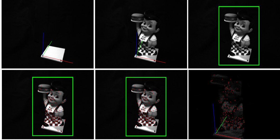
Figure 3.1: The database of features for the object is generated during a training phase. Beginning with the top row, far left, the training phase begins by establishing a set of coordinate axes for the object using a calibration platform. Once established, the object axes is aligned with the axes of the platform (top row, middle image). A bounding box is then defined by the user around the object in the image (top row, far right), where feature extraction is to be applied (bottom row, far left). Features within the bounding box though not part of the image are then removed as shown in the bottom row, middle image (note the features on the white platform have been removed). In the final step, full stereo is applied and nearest-neighbor data association is applied to assign each extracted feature a corresponding 3D point, as defined in the object-reference-frame .
