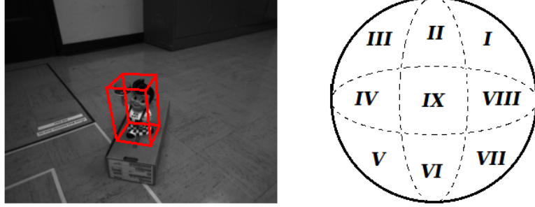
Figure 6.2: The 3D SIFT-based local search and pose estimation process is applied to each of quadrants of the viewing sphere. The diagram on the right depicts the arrangement of search regions while the left image is taken from an experiment where positive detection and pose estimation occurred in quadrant VI .
