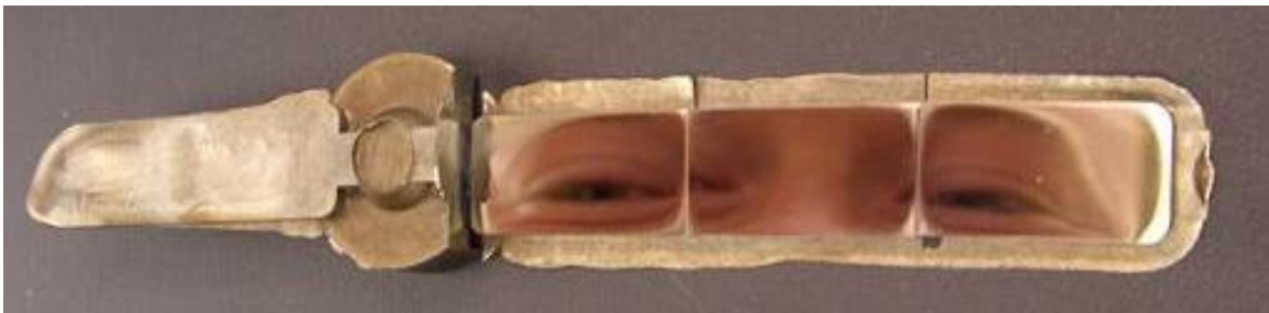
Figure 1.10: Photograph of the polished injection molded part prior to final sectioning for three-point bend testing.
