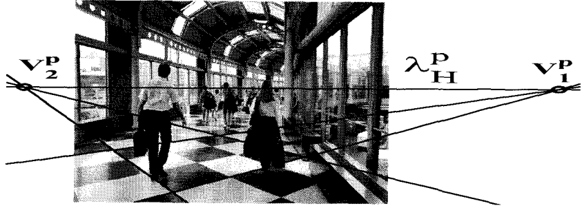
Figure 3.5: Calibration on a natural image: The two sets of parallel lines on the ground floor are used to infer the two vanishing points V_1^P and V_2^P (in pixel coordinates). The line connecting them is the horizon line \lambda_H^P attached to the plane. The image is 341 \times 510 pixels.
