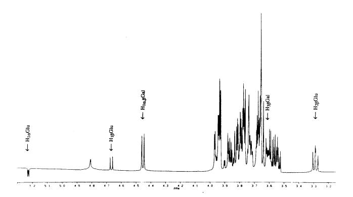
Figure 10. The effect of lactose binding sites on the lactose <sup>1</sup>H NOE difference spectrum. Shown is the off resonance and NOE difference spectra of a) lactose and b) lactose in the presence T206 membranes. For both (A) and (B), the difference spectrum is scaled relative to the off resonance spectrum by a factor of four. Lactose concentration 13 mM (A,B) and protein concentration 3.3 mg/ml (B); 25 °C
