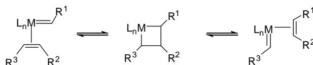
**Figure 1.1.** General mechanism of olefin metathesis.
