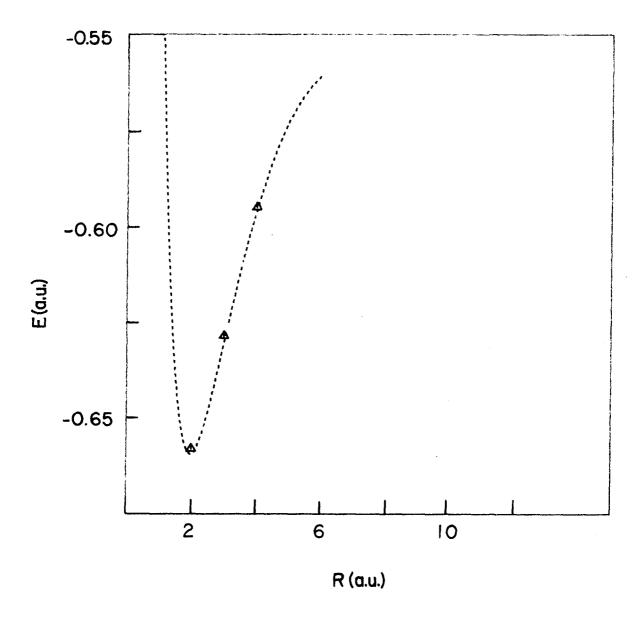
Fig. 32. Total energies for the 3  $^3\Sigma_g^+$  state of  $H_2$  (called g): short dashes, CI (Ref. 37); triangles, present calculation (18 basis functions).
