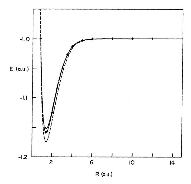
Fig. 10. Total energies for the 1  $^{1}\Sigma_{g}^{+}$  state of H<sub>2</sub> (called X): long dashes, G1 (Ref. 31); medium dashes, exact (Ref. 32); solid line and crosses, present calculation (16 basis functions).
