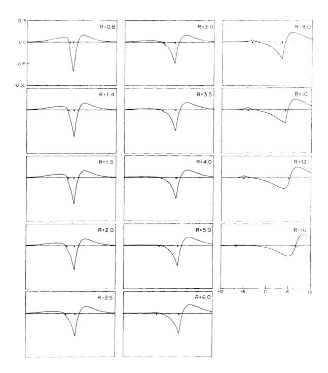
Fig. 26.  $\varphi_{\rm b}$  orbitals for the 1  $^3\Sigma_{\rm g}^+$  state of H<sub>2</sub>, PGVB (16 basis functions).
