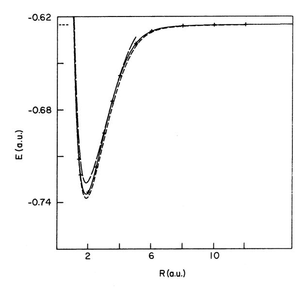
Fig. 27. Total energies for the 1  $^3\Sigma_g^+$  state of  $H_2$  (called a); long dashes, limited CI (Ref. 44), medium dashes, exact (Ref. 40b); solid line and crosses, present calculation (16 basis functions).
