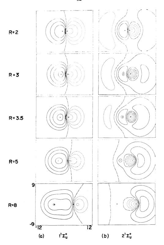
Ref. 21.  $\varphi_{\rm b}$  orbitals for H<sub>2</sub>, PGVB (16 basis functions) contours 0,  $\pm$  0.01,  $\pm$  0.02,  $\pm$  0.04,  $\pm$  0.08.
