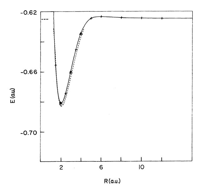
Fig. 35. Total energies for the 2  $^3\Sigma_{\rm u}^+$  state of H<sub>2</sub> (called e); short solid arc from R = 1.9 to R = 2.1, CI (Ref. 36); short dashes, RKR (Ref. 45); solid line and crosses, present calculation (16 basis functions); triangles, present calculation (18 basis functions).
