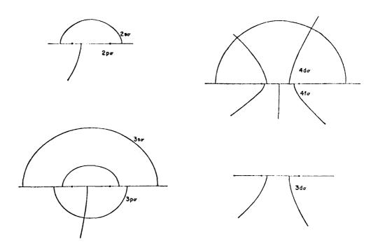
Fig. 5. The nodal surfaces for the first eight  $\sigma$  states of HeH<sup>+2</sup> at R = 2 a.u., from Ref. 27.
