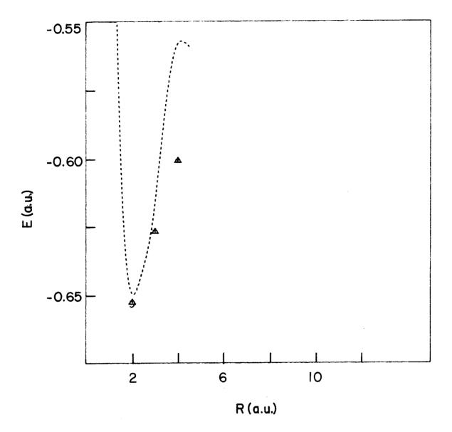
Fig. 18. Total energies for the 4  $^{1}\Sigma_{g}^{+}$  state of H<sub>2</sub> (called G): short dashes, CI (Ref. 33b); short solid arc from R = 1.9 to R = 2.1, CI (Ref. 36); triangles, present calculation (18 basis functions).
