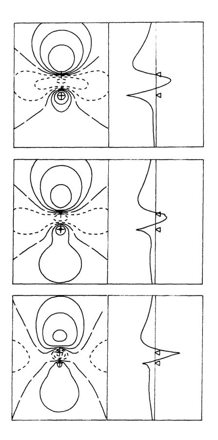
R = 2, 3, 4; horizontal scale ± 12 a.u.; vertical scale contour plot ± 9 a.u.; line plot  $\varphi_{\rm b}$  orbitals for the 2  $^3\Sigma_{\rm g}^+$  state of H<sub>2</sub>; PGVB (18 basis functions); from left to right  $\pm$  0.15 amplitude; contours 0,  $\pm$  0.01,  $\pm$  0.02,  $\pm$  0.04,  $\pm$  0.08. Fig. 29.
