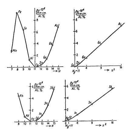
Fig. 1. Increase in the resistance of copper due to one atomic per cent of various metals in solid solution.
