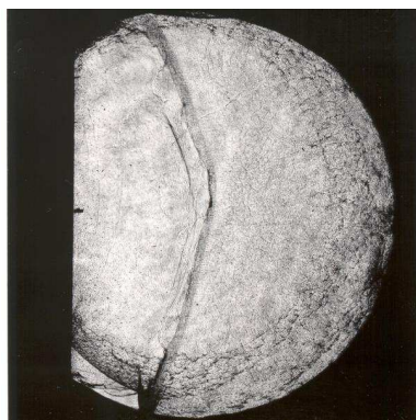
Figure M.182: Shot 208, 0.222 \text{ C}_2\text{H}_6 + 0.778 \text{ O}_2 , P_0=40 \text{ kPa} , T_0=295 \text{ K} . Delays: \Delta t(\text{P3-schl}) 190.2 \mu\text{s} ; \Delta t(\text{TEP-schl}) 62.32 \mu\text{s} . Schlieren image height 150 mm.
