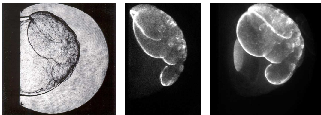
Figure M.197: Shot 223, 0.222 \text{ C}_2\text{H}_6 + 0.778 \text{ O}_2 , P_0=42.5 \text{ kPa} , T_0=298 \text{ K} . Delays: \Delta t(\text{P3-PLIF}) 161.36 \mu\text{s} ; \Delta t(\text{TEP-PLIF}) 33.63 \mu\text{s} . Delays: \Delta t(\text{P3-chem}) 156.36 \mu\text{s} ; \Delta t(\text{TEP-chem}) 28.63 \mu\text{s} . Schlieren image height 150 mm, Chemiluminescence image 1 height 140 mm, Chemiluminescence image 2 height 140 mm.
