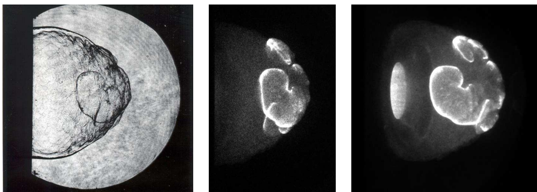
Figure M.200: Shot 227, 0.222 \text{ C}_2\text{H}_6 + 0.778 \text{ O}_2 , P_0=42.5 \text{ kPa} , T_0=298 \text{ K} . Delays: \Delta t(\text{P3-PLIF}) 160.36 \mu\text{s} ; \Delta t(\text{TEP-PLIF}) 32.63 \mu\text{s} . Delays: \Delta t(\text{P3-chem}) 156.36 \mu\text{s} ; \Delta t(\text{TEP-chem}) 28.63 \mu\text{s} . Schlieren image height 150 mm, Chemiluminescence image 1 height 140 mm, Chemiluminescence image 2 height 140 mm.
