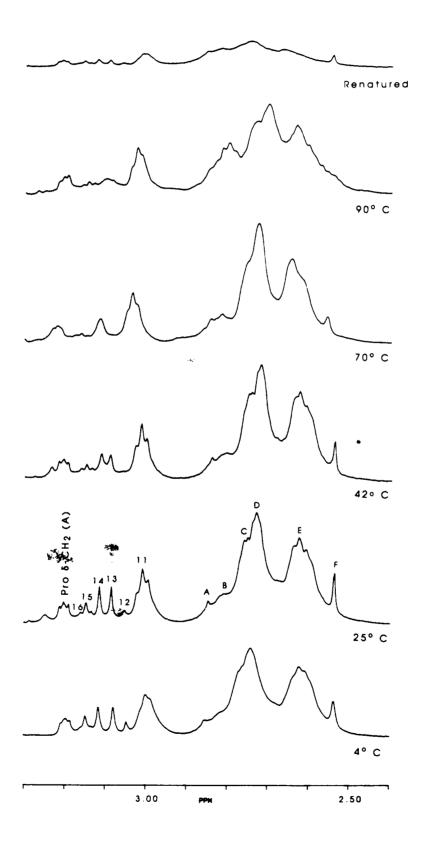
Figure 3: Temperature Dependence of <sup>31</sup>P NMR Spectra of BDPP at pH 7.0.
