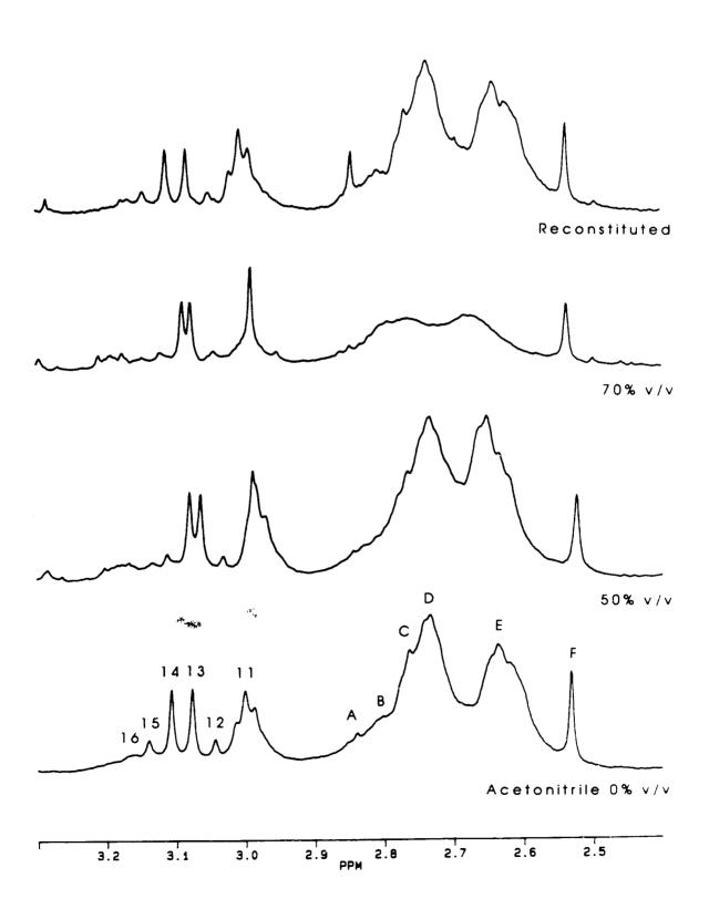
Figure 7: Solvent Effects on the <sup>31</sup>P NMR Spectra of BDPP, pH 7.0.
