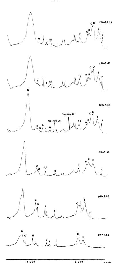
Figure 3: <sup>1</sup>H NMR 500 MHz Spectra of BDPP as a Function of pH.
