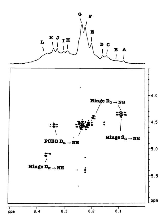
Figure 3: "Clean" <sup>1</sup>H - <sup>1</sup>H NMR HOHAHA (500.138 MHz) spin-lock correlation spectroscopy of α-CH fingerprint region of INTERVI (1.2 mM) in D2O at (A) pH 7.08, low ionic strength, divalent-cation depleted (B) as in A, but at pH 2.15, (C) pH 7.16, in the presence of 17.5 mM <sup>113</sup>Cd (II)
