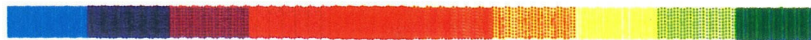
Figure 6-9. Color code for the X-Y data plots. The scale is 2 and 1/3 dB per color. Power increases from left to right. Green colors represent large RF power.
