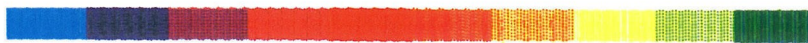
Figure 7-29. Color code for the data plots. The scale is linear with lowest to highest going from left to right. The upper bound of the lowest color is -7.4\text{mV} (across the input resistance of the amplifier). The upper bounds of the next eight colors in mV are 2.6, 12.6, 22.6, 32.6, 42.6, 52.6, 62.6 and 72.6. The lower bound of the largest color is 72.6\text{mV} .
