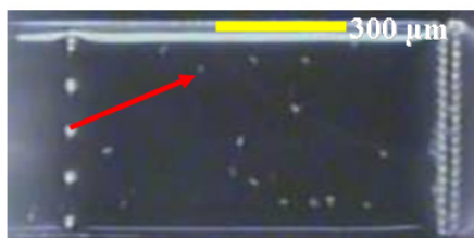
Figure 6-3. Prorocentrum gracile inside the Parylene culture chamber. Arrow indicates one of the cells.
