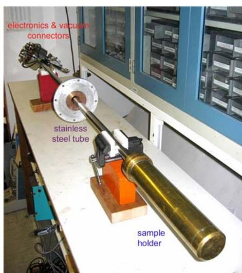
**Figure 7.1** The “dipper” used to conduct low-temperature experiments on (Ga,Mn)As. The length is around 2 meters, and everything underneath the flange is immersed in a liquid helium cryostat. The brass sample holder fits inside a 3-axis superconducting solenoid.
