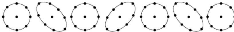
Figure 2.2: Illustration of the effect of a gravitational wave with cross polarization on a ring of test particles when the direction of propagation of the gravitational wave is orthogonal to the plane of the particles.
