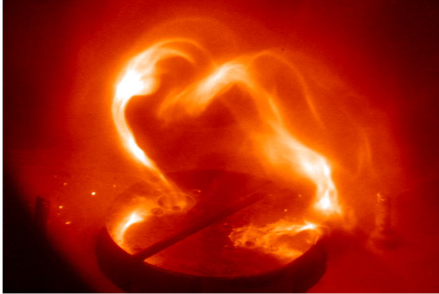
Figure 5.1: A photograph of a prominence-like configuration produced in a laboratory experiment using the modified spheromak technology (image courtesy of J.F. Hansen and P.M. Bellan)
