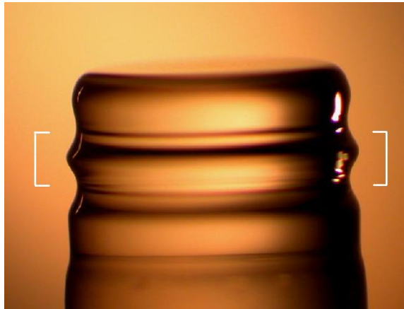
Figure 4.1: CaF 2 cavity with a record Q factor of (6.3 \pm 0.8) \times 10^{10} , 5.5 mm in diameter. White brackets show the area of WGM localization.
