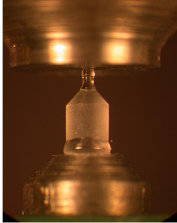
Figure 3.10: \text{MgF}_2 resonator is deformed along its axis with a piezo element. Resonator diameter is 500\ \mu\text{m} .
