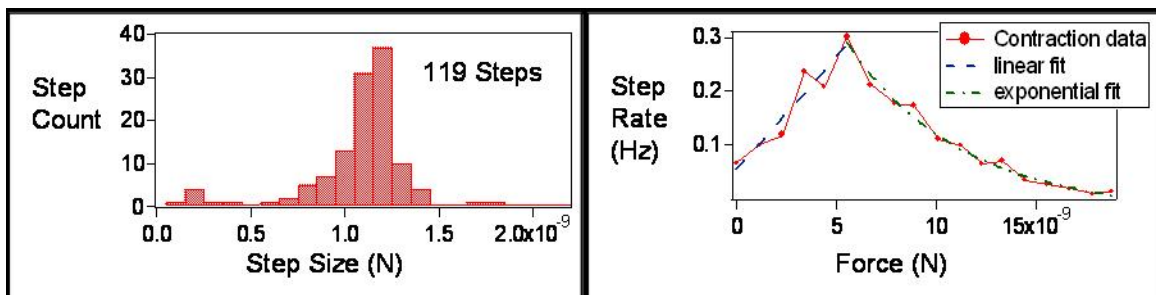
Figure 35. Examples of the statistical and dynamic data which can be obtained with SCPFM. Above left is a histogram of step sizes from 3 Cytochalasin D induced relaxation and contraction cycles on a single cell.
