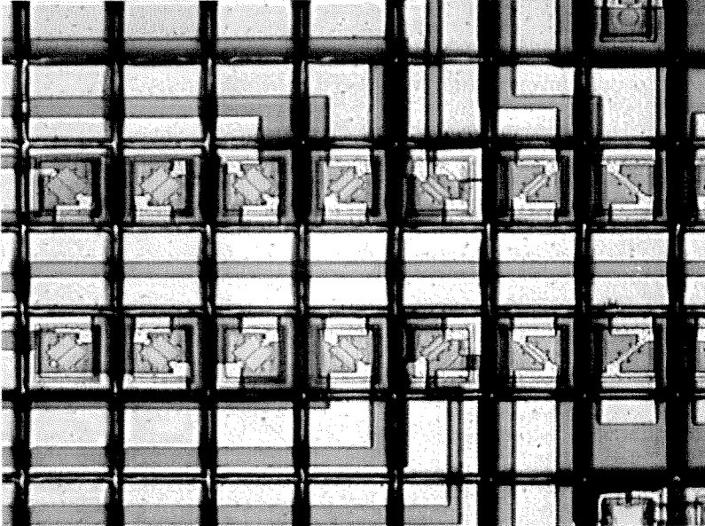
Figure 3.11 Two rows of shear-stress sensors on silicon islands.
