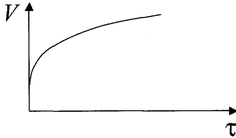
Figure 1.15 Typical voltage output of shear-stress sensor at CT mode.
