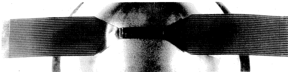
Figure 2.11 A sensor skin solder-bonded to a flexible PCB with a dome underneath.
