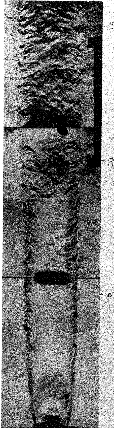
Figure 10. Composite Photograph of Flame Spreading from 1 inch Diameter Flameholder; \phi = 1.0 , 300 ft/sec Mixture Velocity
