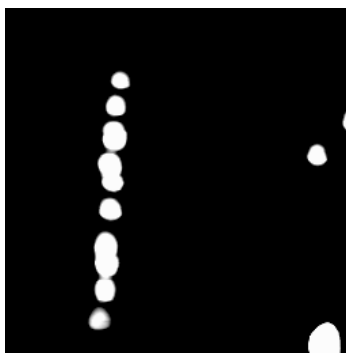
Figure 5-3: Atomic force microscopy fabrication of plasmon waveguides (II). Atomic force microscopy scan of a 10 particle plasmon waveguide consisting of 30 nm colloidal Au particles. The scan shows a 1 \times 1 \mu\text{m}^2 area after the randomly deposited particles were pushed in place using the AFM tip (courtesy of Sheffer Meltzer).
