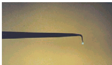
Figure 6-5 (color): Nanonics NSOM tip drawn from a conventional optical fiber that has been tapered down and bent to enable an AFM-type normal force feedback. The light emanating from the aperture in illumination mode can be seen (courtesy of Nanonics Imaging Ltd).
