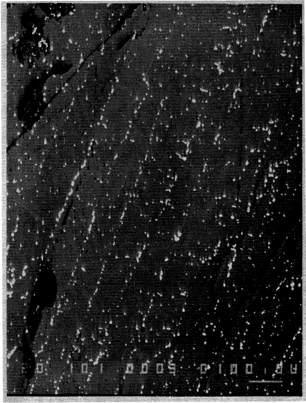
Figure IV-2b SEM micrograph of annealed LaNi 4.5 Ge 0.5 ingot.
