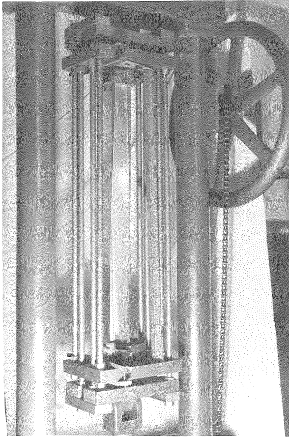
View of Testing Machine Showing Compression Cage, Method of Mounting, and Typical Torsion Failure of the Specimen
