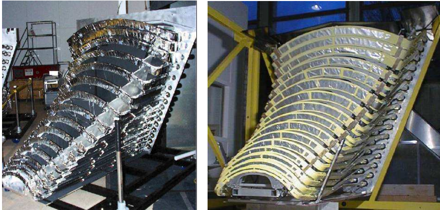
Figure 2-10: Left NA, right FR octants with the 16 pairs of arc shaped iso- Q^2 FPD segments each.
