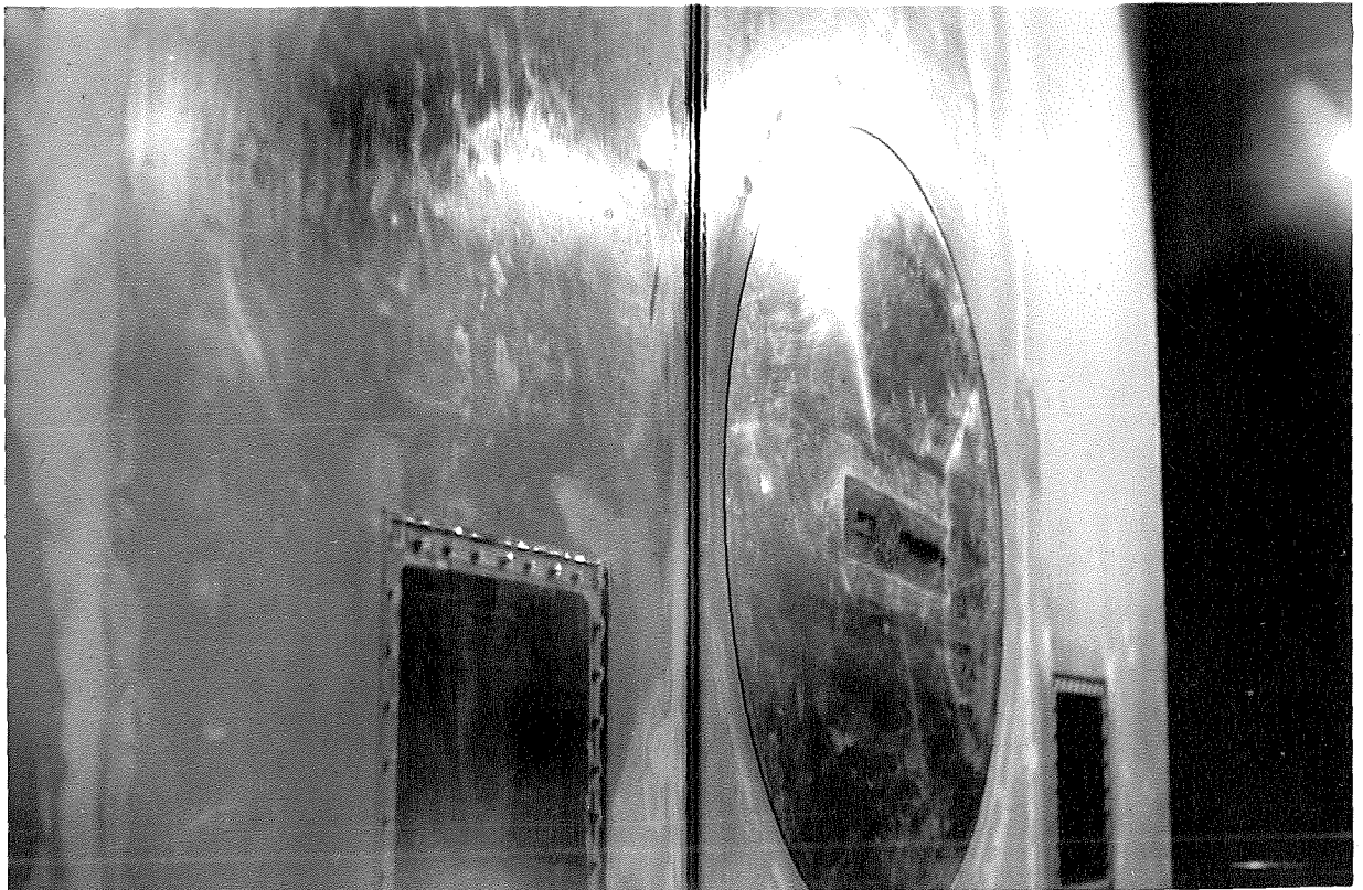
Photo 2. Front view showing roughness strip mounted ahead of end plate.
