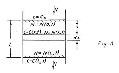
In the portion of the bed between x and x + dx, indicated in Fig. A, the rate of removal of material from the air stream with respect to time would be
