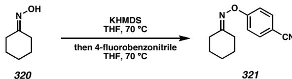
**O-Aryloxime 321.** In the glovebox, a flamedried round-bottom flask under argon was charged with KHMDS (484.1 mg, 2.43 mmol) and removed from the glovebox. A solution of cyclohexanoxime (**320**) (250 mg, 2.21 mmol) in THF (20 mL) was added. The reaction was fitted with a reflux condenser and heated to 70 °C for 1 h. Then, a solution of 4-fluorobenzonitrile (267.7 mg, 2.21 mmol) in THF (5 mL) was added.
