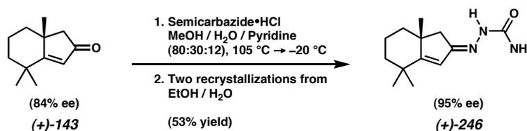
**Bicyclic Semicarbazone (+)-246.** A round-bottom flask containing the scalemic bicyclic enone (+)-**143** (3.04 g, 17.06 mmol, 1.00 equiv, 84% ee) was charged with MeOH (48.6 mL), H<sub>2</sub>O (18.2 mL), and pyridine (7.30 mL). Semicarbazide hydrochloride (3.42 g, 30.7
