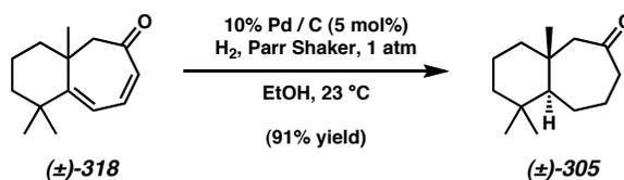
**Cycloheptanone (±)-305.** A Parr flask was charged with 10% w/w Pd/C (150 mg, 0.142 mmol), followed by a solution of cycloheptadienone (±)-318 (580 mg, 2.84 mmol) and
