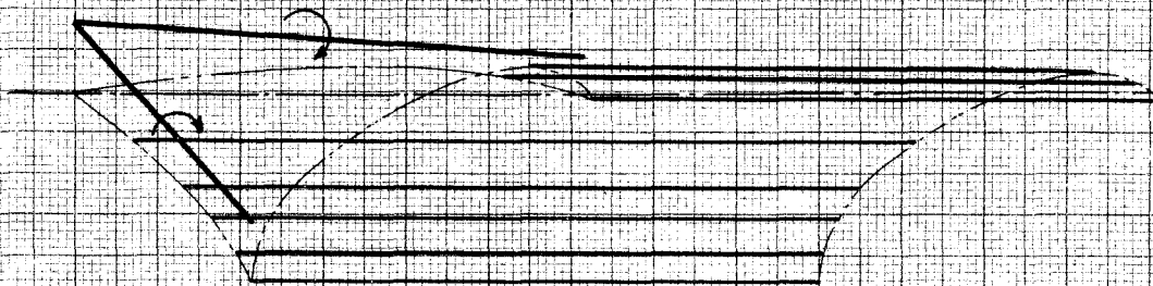
Figure (13) - Distorted Shape of the Vortex Pattern as Assumed for Use in Making Final Downwash Calculations
