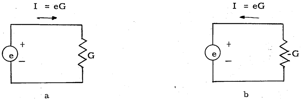
Figure 5. Direction of Current Flow in Positive and Negative Conductances
