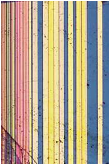
Figure 1.5: 90° domain patterns in \text{PbTiO}_3 obtained by using polarized light microscopy. The area imaged is about 2.5 \text{ mm} \times 1.2 \text{ mm} .
