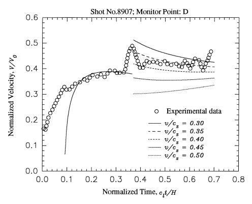
Figure 4.4: Analytical simulation of the experimental measurement at monitoring point D by Prakash and Clifton (1992), shot No. 8907. Before crack initiation, full field expression for the particle velocity is used. After crack initiation, three-term transient asymptotic representation given in equation (4.3.2) with constant crack-tip speed has been used.
