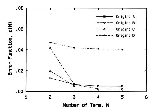
Figure 5.6: Variation of the error function  $\epsilon(N)$  with the term number N for different locations of the origin.
