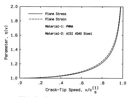
Figure 6.2: Velocity dependence of mismatch parameter  $\eta$  for plane stress and plane strain.
