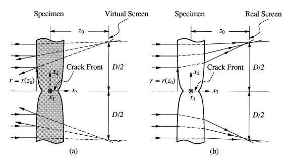
Figure 5.1: Caustic formation in (a) reflection, (b) transmission.
