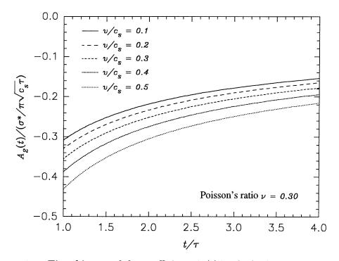
Figure 3.5: Time history of the coefficient  $A_2(t)$  in the higher order transient asymptotic expansion for the moving crack under stress wave loading conditions.
