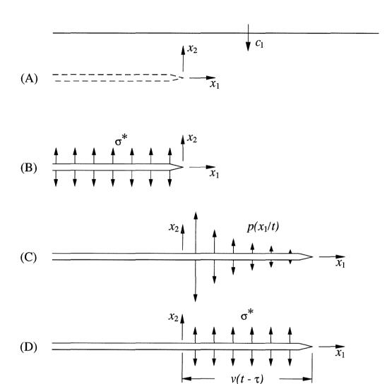
Figure 3.2: Schematic representation of the various boundary value problems considered in constructing the solution for constant speed crack growth under stress wave loading conditions.
