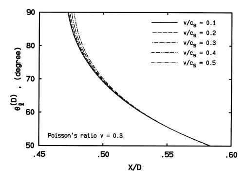
**Figure 5.10**: Value of the parameter  $\theta_l^{(D)}$ , solved from equation (5.3.20), versus the ratio X/D, for different crack-tip speeds.
