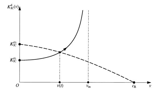
Figure 4.6: Schematic description of dynamic crack initiation and propagation.
