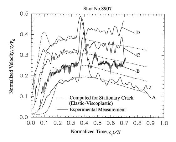
Figure 4.3: Experimental and numerical predicted (stationary crack) velocity-time profiles at four different monitoring points, from Prakash and Clifton, 1992.
