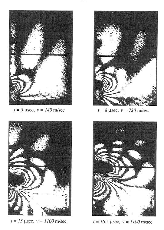
Figure 6.13: Selected sequence of CGS interferogram of a growing crack in a one point bend interfacial gas gun experiment. (Only PMMA side of PMMA/steel specimen is shown)
