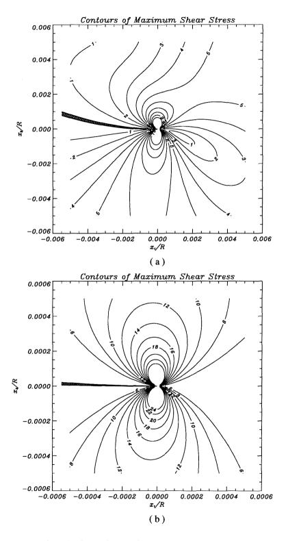
Figure 2.2: Simulated photoelastic fringe patterns surrounding the tip of a crack propagating along a curved path, (a) larger observation region, (b) observation in the region very close to the crack-tip.
