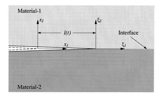
Figure 6.1: Schematic of dynamic growth of a crack along the bimaterial interface.
