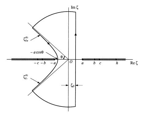
Figure 3.9: Distortion of the integral contour to evaluate the inversion of  $G(\zeta, x_2, s)$ .
