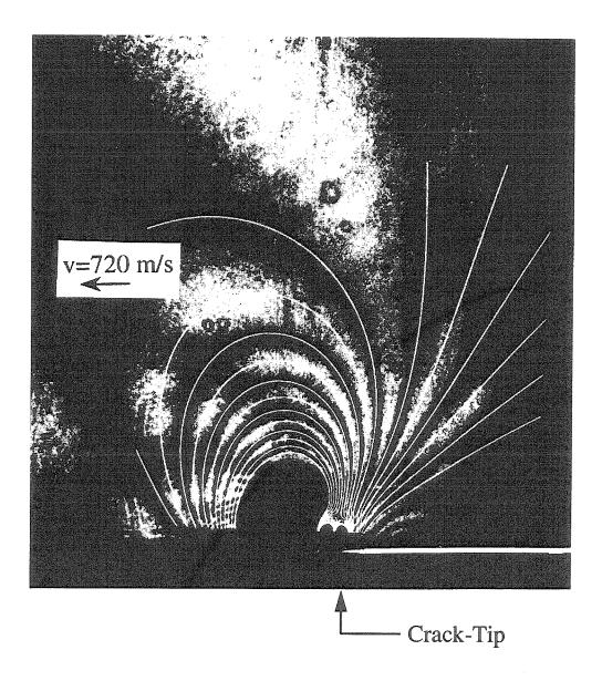
Figure 6.16: Comparison between the CGS fringe pattern and the fitted higher order transient stress field, equation (6.7.10), for a propagating crack in a PMMA/steel interface.
