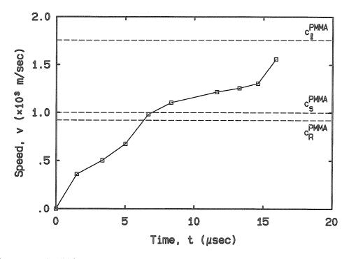
Figure 6.17: Velocity time history for the experiment shown in Figure 6.18.
