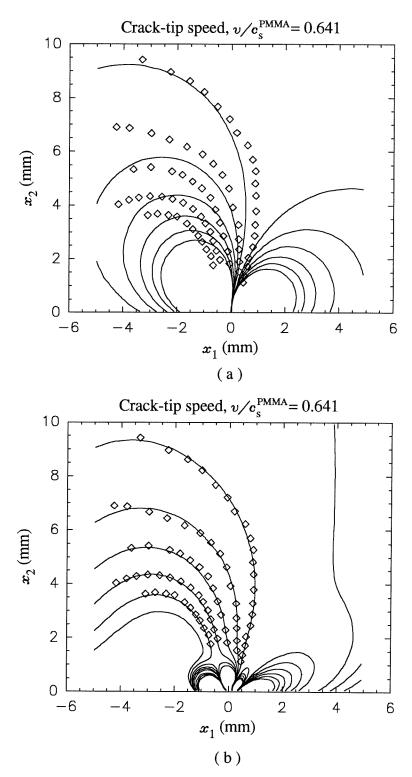
Figure 6.11: Comparison of digitized data points from the interferogram corresponding to  $t = 9.5\mu$ sec in FIGURE 6.8 with, (a) a  $K^d$ -dominant fit, equation (6.7.9); (b) a higher order transient analysis fit, equation (6.7.10). (Crack lies along the negative  $x_1$ -axis)
