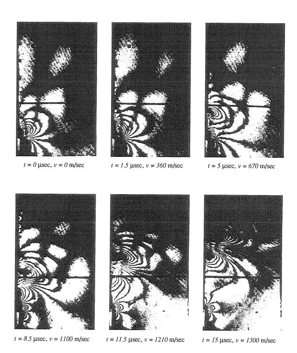
Figure 6.18: Selected sequence of CGS interferograms of a growing crack in a one point bend interfacial gas gun experiment. (A blunt starter notch was used)
