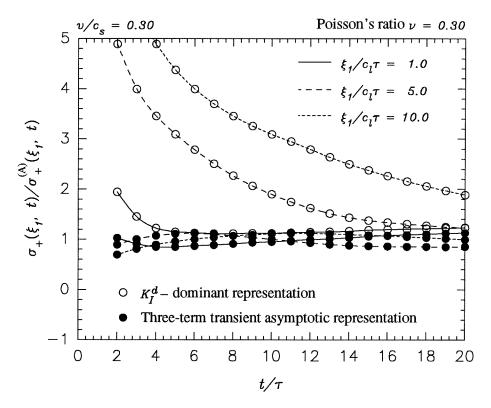
**Figure 3.8**: Comparison of the time histories of the  $K_I^d$ -dominant and the higher order transient asymptotic representation of normal traction ahead of the moving crack-tip at different distances from the crack-tip.
