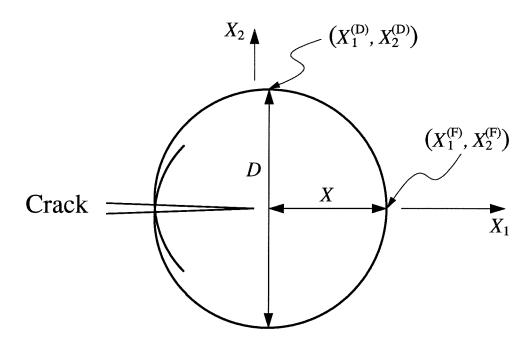
**Figure 5.2**: Evaluation of the dynamic stress intensity factor  $K_I^d(t)$  by measuring two geometrical dimensions, D and X.
