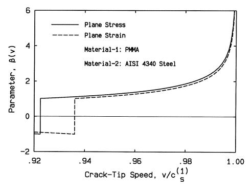
Figure 6.4: Velocity dependence of mismatch parameter  $\beta$  for plane stress and plane strain at the vicinity of the shear wave speed of PMMA.
