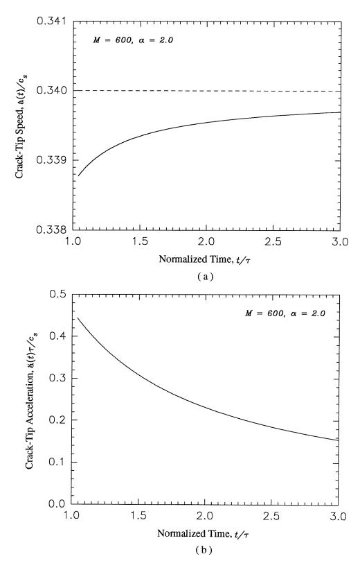
Figure 4.7: Time histories of the crack-tip speed (a), and crack-tip acceleration (b), where  $\alpha = 2.0$  and M = 600 have been chosen.
