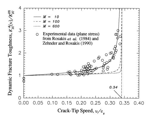
Figure 4.5: Comparison of the relationship between the dynamic fracture toughness and the crack-tip speed. Different lines represent the prediction using equation (4.4.8) and circles are the experimental results obtained by Rosakis *et al.* (1984) and Zehnder and Rosakis (1990).
