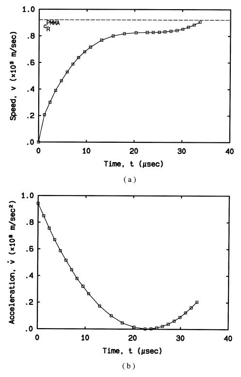
Figure 6.9: Velocity, (a) and acceleration, (b) time histories for the experiment shown in Figure 6.8.
