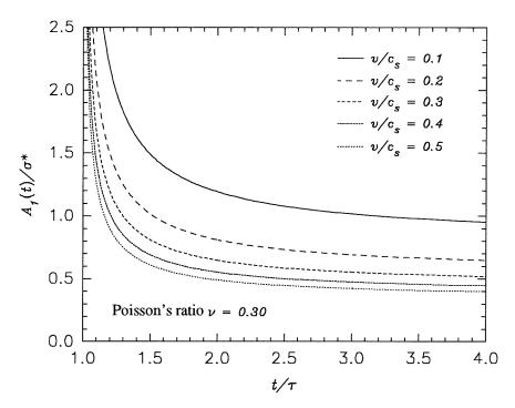
Figure 3.4: Time history of the coefficient  $A_1(t)$  in the higher order transient asymptotic expansion for the moving crack under stress wave loading conditions.
