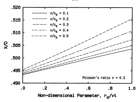
Figure 5.11: Ratio X/D versus the non-dimensional parameter  $r_0/vt$  for different crack-tip speeds.
