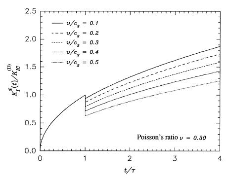
Figure 3.3: The dynamic stress intensity factor history for the stationary and propagating crack under stress wave loading conditions.
