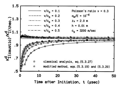
**Figure 5.13**: Variation of the ratio  $K_{I(caustic)}^d/K_{I(theo.)}^d$  with the time after crack initiation for different crack-tip speeds. The material parameters correspond to 4340 steel.
