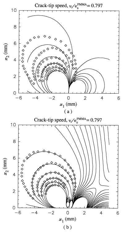
Figure 6.12: Comparison of digitized data points from the interferogram corresponding to  $t = 23\mu$ sec in Figure 6.8 with, (a) a  $K^d$ -dominant fit, equation (6.7.9); (b) a higher order transient analysis fit, equation (6.7.10). (Crack lies along the negative  $x_1$ -axis)
