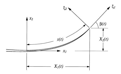
Figure 2.1: Crack growing along a smooth curved path under two-dimensional conditions. The instantaneous crack-tip position is  $x_1 = X_1(t)$ ,  $x_2 = X_2(t)$ , and the instantaneous crack-tip speed is v(t) in the local  $\xi_1$ -direction.
