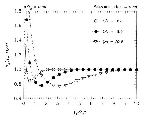
Figure 3.6: Distribution of normal traction ahead of the moving crack-tip at different instants of time.
