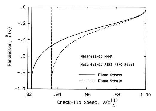
Figure 6.6: Velocity dependence of the real part of mismatch parameter  $\epsilon$  for plane stress and plane strain at the vicinity of the shear wave speed of PMMA.
