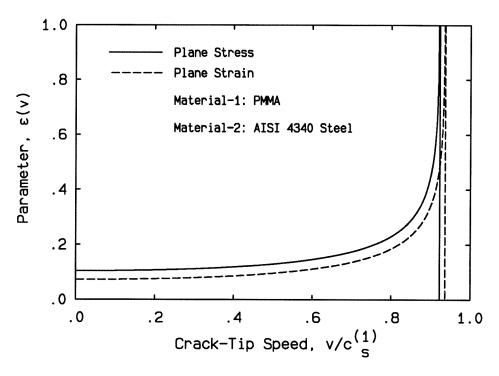
Figure 6.5: Velocity dependence of mismatch parameter  $\epsilon$  for plane stress and plane strain.
