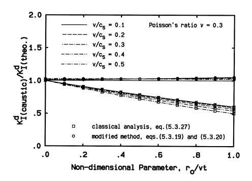
Figure 5.12: Comparison of the dynamic stress intensity factor inferred from the modified method and the classical analysis for different values of  $r_0/vt$ , and for different crack-tip speeds.
