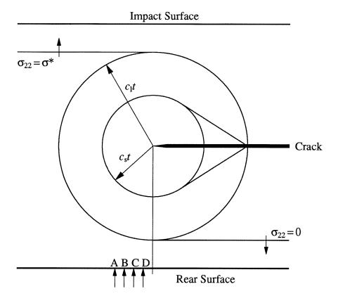
Figure 4.1: Wavefronts for the diffraction of a planar wave by a semi-infinite crack.
