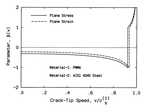
Figure 6.3: Velocity dependence of mismatch parameter  $\beta$  for plane stress and plane strain.
