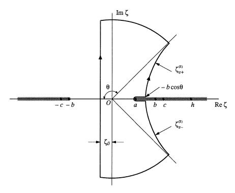
Figure 3.10: Distortion of the integral contour to evaluate the inversion of  $W(\zeta, x_2, s)$ .
