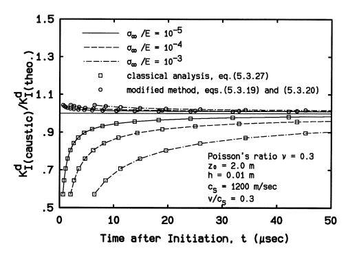
Figure 5.14: Variation of the ratio  $K_{I(caustic)}^d/K_{I(theo.)}^d$  with the time after crack initiation for different load levels,  $\sigma_{\infty}/E$ .
