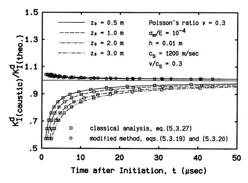
**Figure 5.15**: Variation of the ratio  $K_{I(caustic)}^d/K_{I(theo.)}^d$  with the time after crack initiation for varying experimental parameter  $z_0$ .
