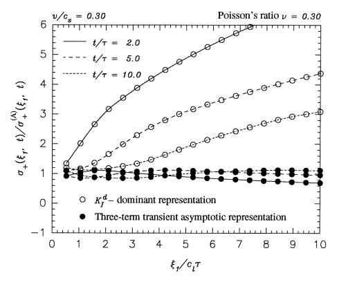
**Figure 3.7**: Comparison of the  $K_I^d$ -dominant and the higher order transient asymptotic distributions of normal traction ahead of the moving crack-tip at different instant of time after crack initiation.
