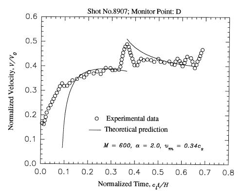
Figure 4.8: Analytical simulation of the experimental measurement at monitoring point D by Prakash and Clifton (1992), shot No. 8907. Before crack initiation, full field expression for the particle velocity is used. After crack initiation, three-term fully transient asymptotic representation given in equation (4.3.2) has been used.
